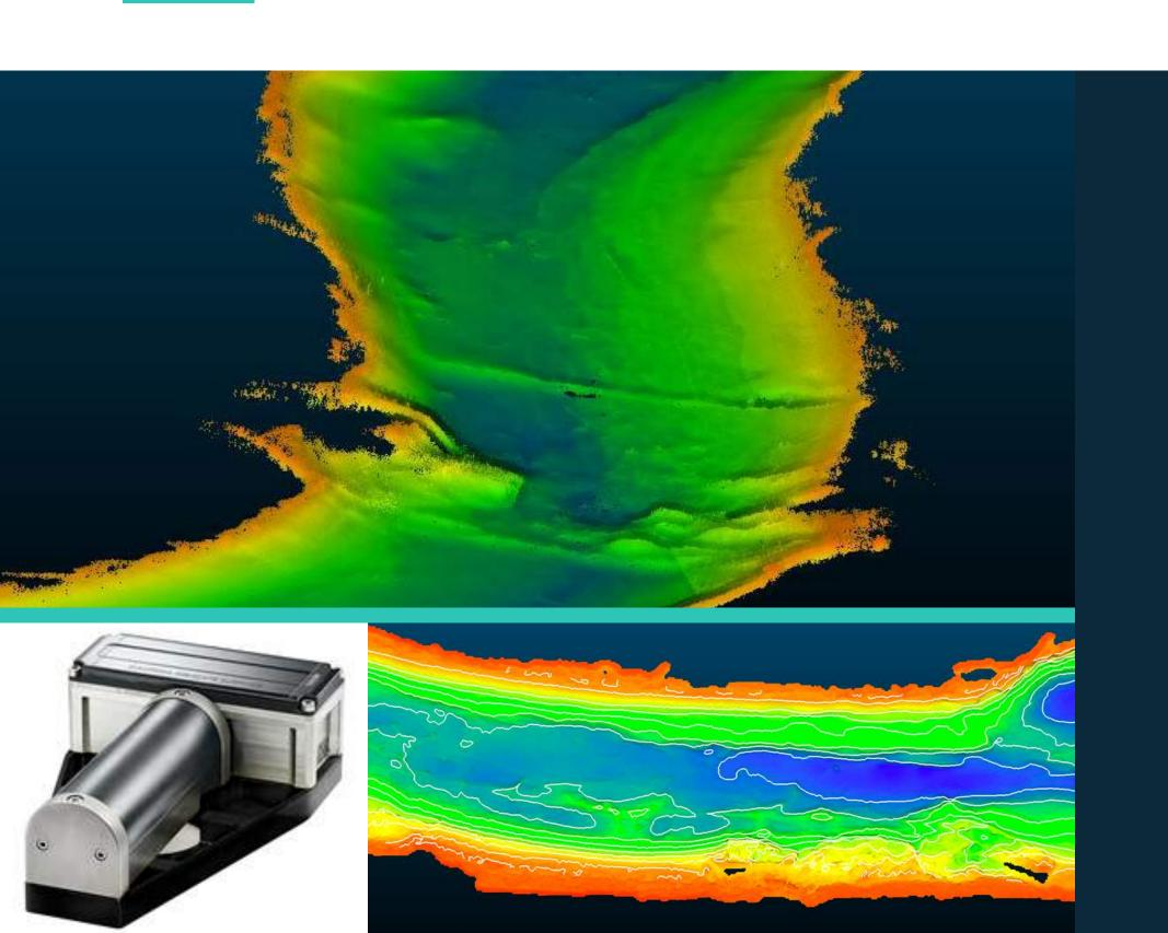
A core specialism of SEP Hydrographic is the use of an of acoustic sensors to map the depth and form of the seabed including coastal areas, ports, harbours, rivers lakes and inland waterways.
